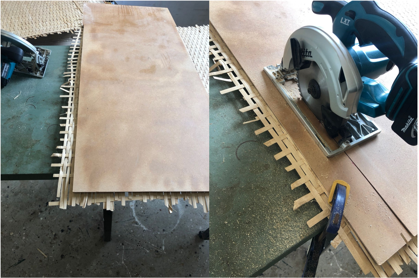
Figure 36. A sacrificial cover sheet on top of the mat helps to stabilize individual strands in the mat and results in cleaner sample edges when a circular saw is used.
