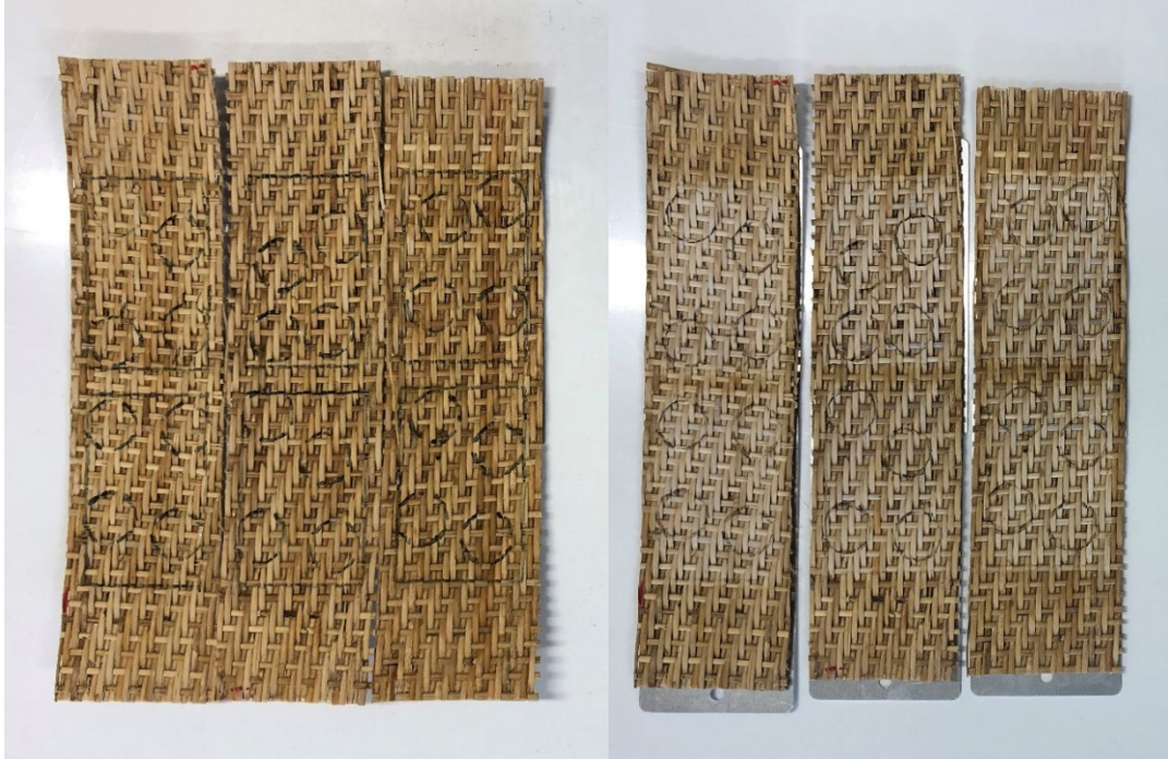
Figure 21. Mats #3 (from left: 3.3.3, 3.3.2, and 3.3.1) after 24 hours (left) and 336 hours (right) of UV exposure.
