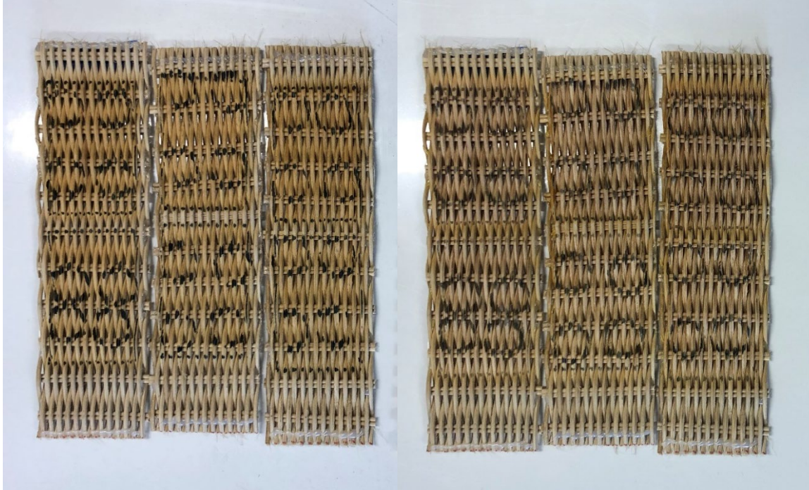
Figure 31. Mats #5 (from left: 5.1.3, 5.1.2, and 5.1.1) after 24 hours (left) and 336 hours (right) of UV exposure.
