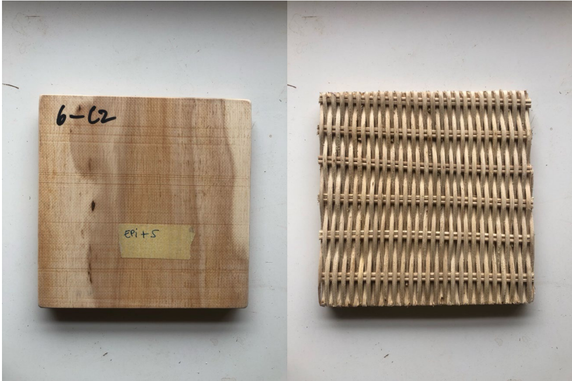
Figure 59. Finished decorative paneling prototype - FSC certified rattan on rubberwood and eucalyptus K7.
