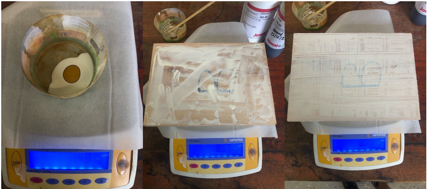
Figure 53. Weighing and preparation for emulsion polymer isocyanate (EPI) application.
