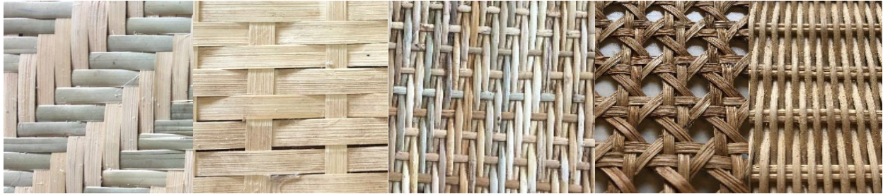
Figure 5. Selected types of mat for the present study. From left to right: Mat #1 (Material: Bamboo), Mat #2 (Bamboo), Mat #3 (Rattan), Mat #4 (Rattan) and Mat #5 (Rattan)
