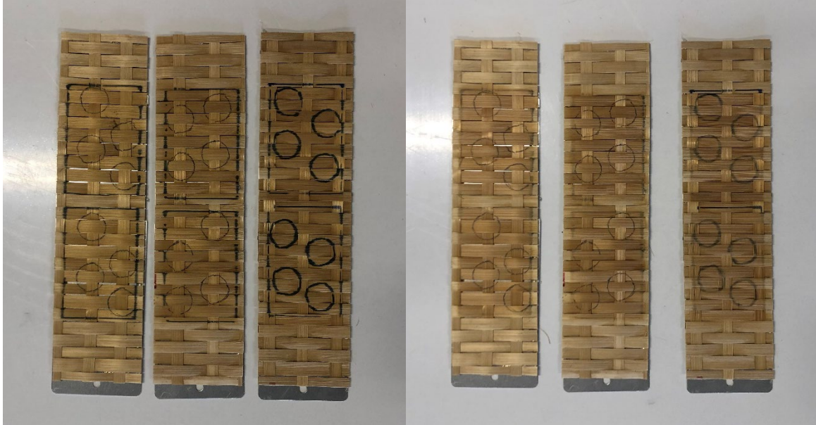
Figure 16. Mats #2 (from left: 2.1.3, 2.1.2, and 2.1.1) after 24 hours (left) and 336 hours (right) of UV exposure.
