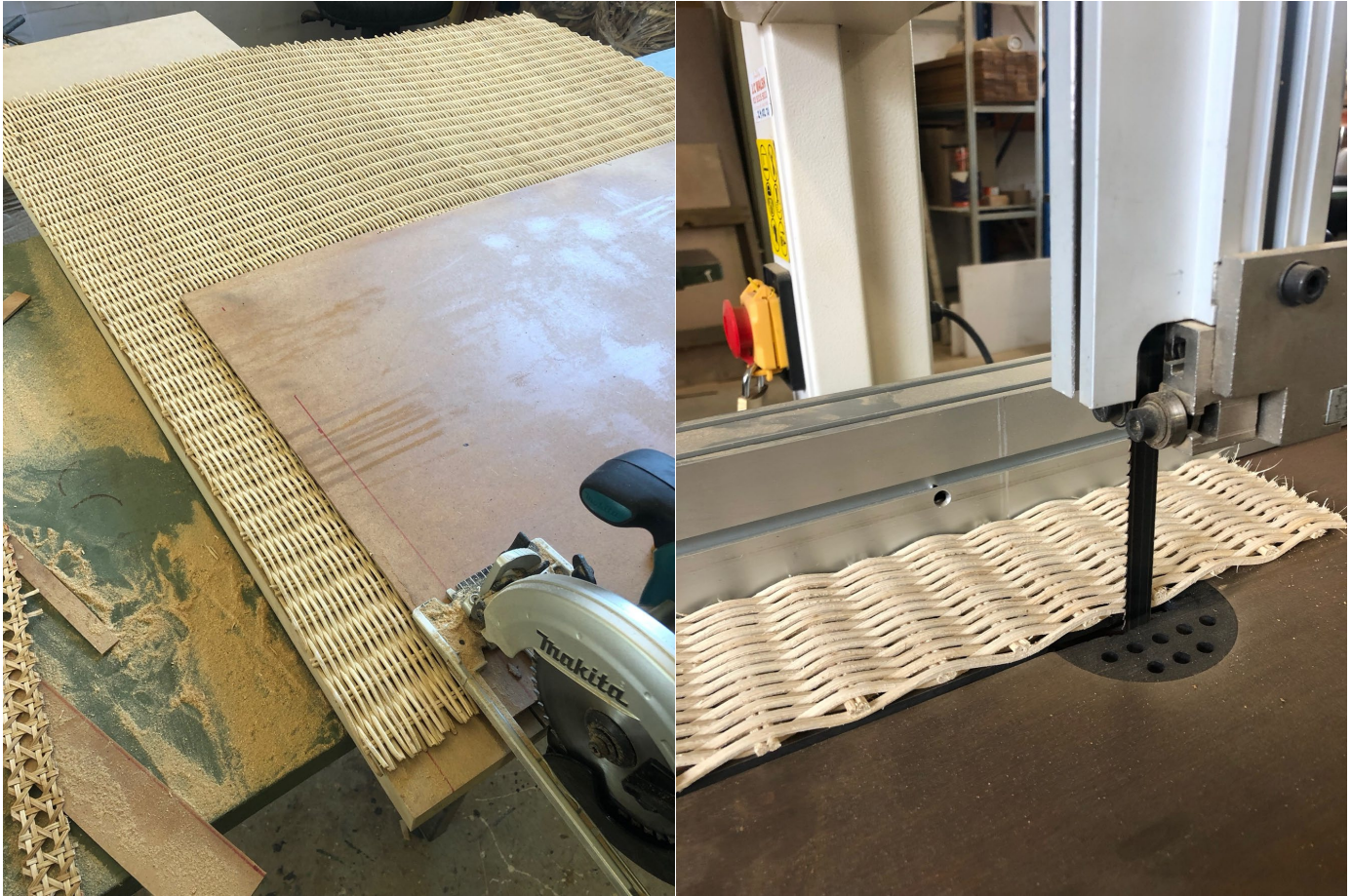
Figure 39. Mat design 5 has a tighter weave and thicker individual strands that machine well with either the sawing equipment (band, circular or table saw)
