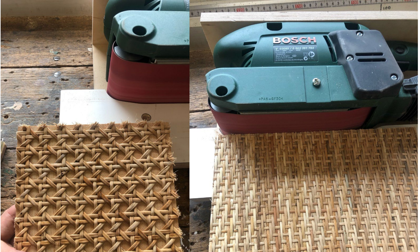
Figure 57. Panel with torn out fibres ready for smoothing on the belt sander.
