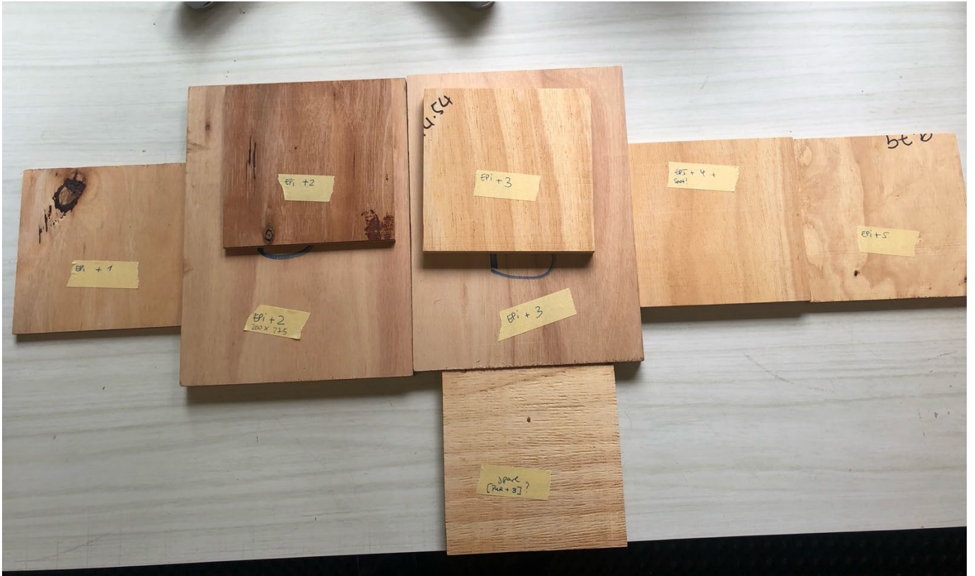
Figure 52. Array of panels to be used as backing layer for the decorative paneling products.
