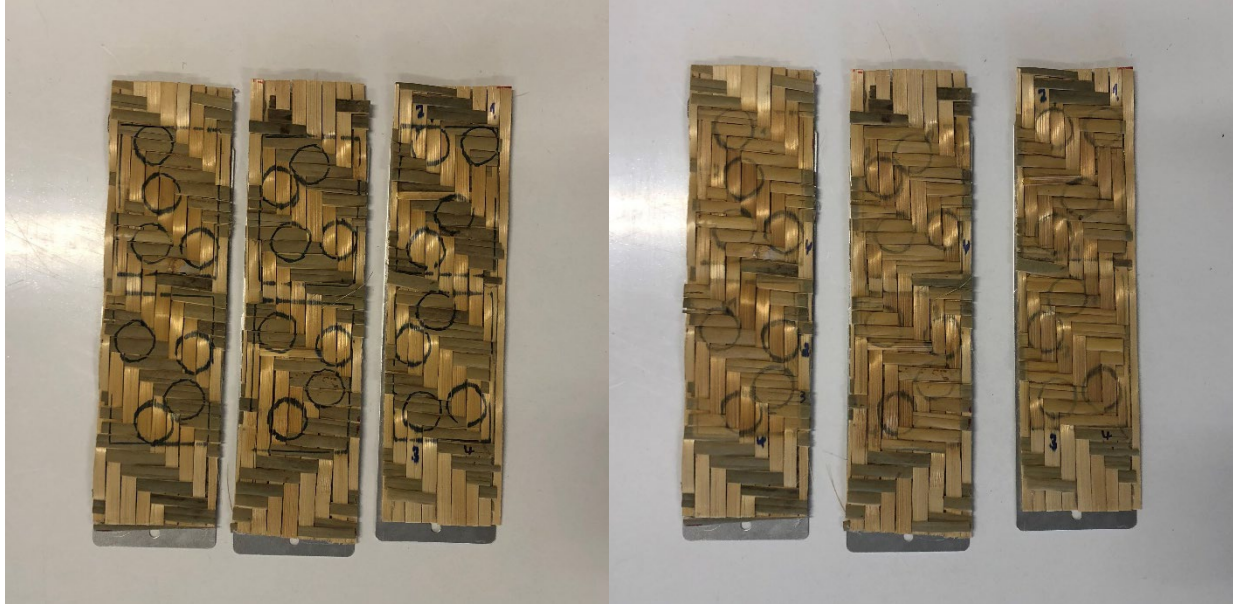
Figure 11. Mats #1 (from left: 1.1.3, 1.1.2, and 1.1.1) after 24 hours (left) and 336 hours (right) of UV exposure.
