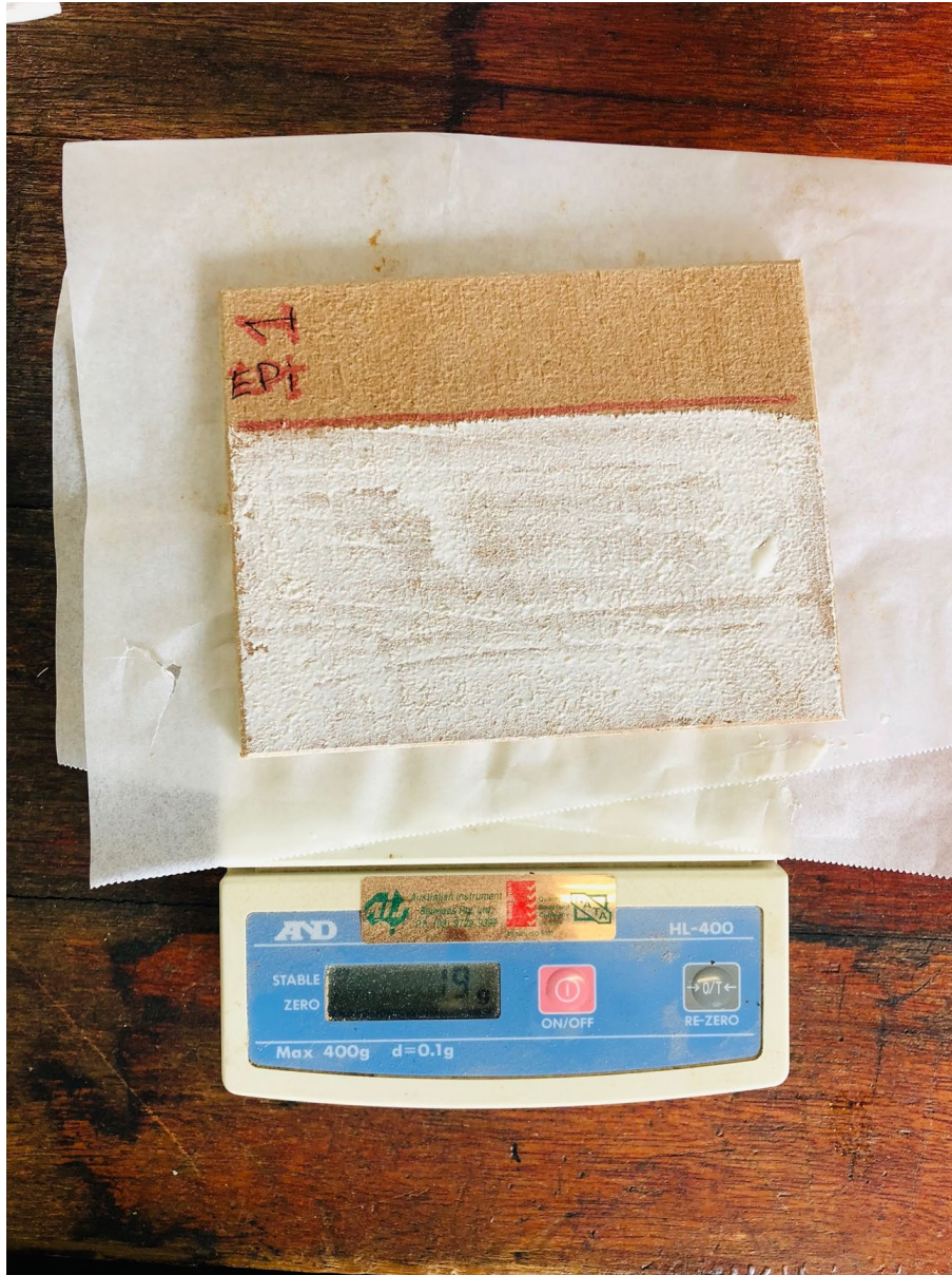
Figure 47. Application of EPI adhesive with flat edge of the spatula.
