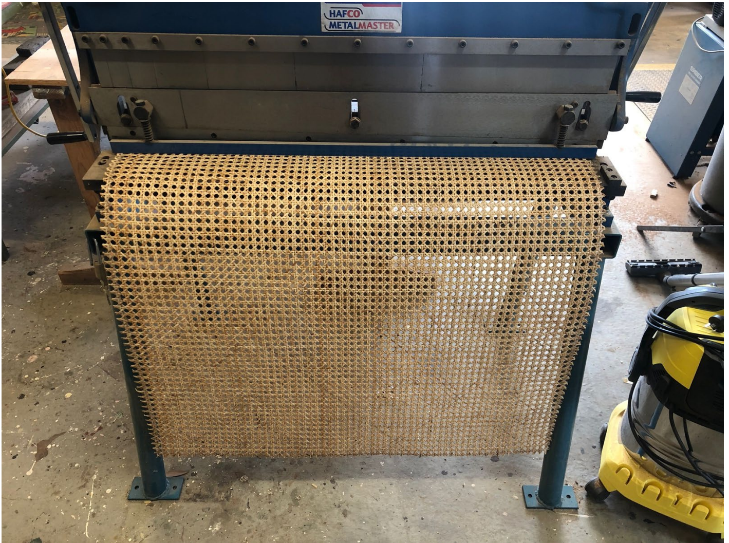
Figure 42. In some cases the width of the mat did not exceed the capacity of the guillotine and the entire sample could be generated using the guillotine alone.
