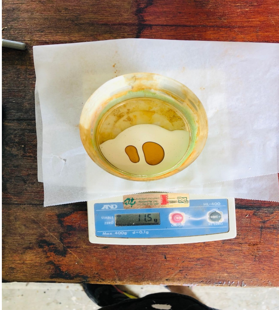
Figure 46. Mixing of 2-component EPI adhesive.
