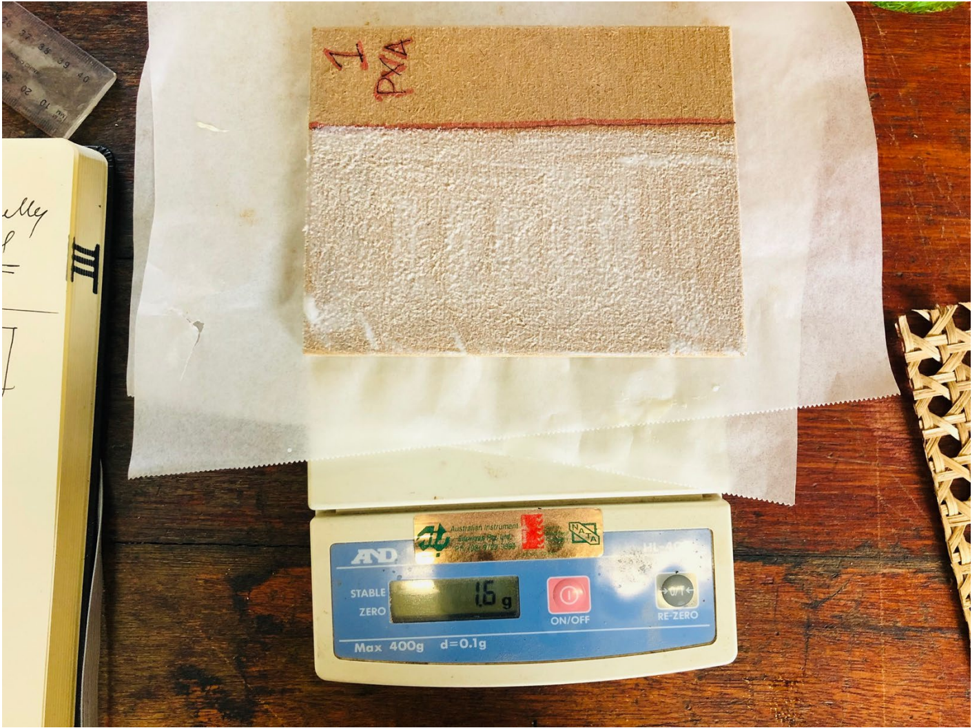
Figure 49. Application of PVA adhesive with flat edge of the spatula.
