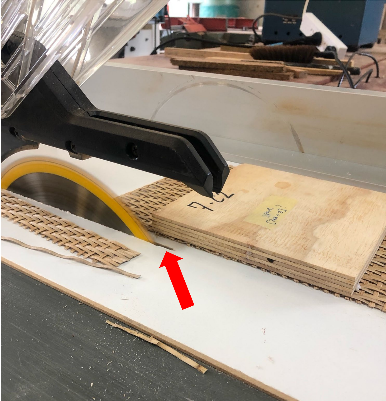
Figure 56. Trimming the mat back to the plywood edge. Notice the reduced gap between table and saw blade using a sacrificial MDF sheet.
