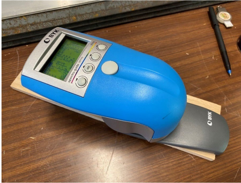
Figure 8. The spectrophotometer used to measure the colour of a sample.
