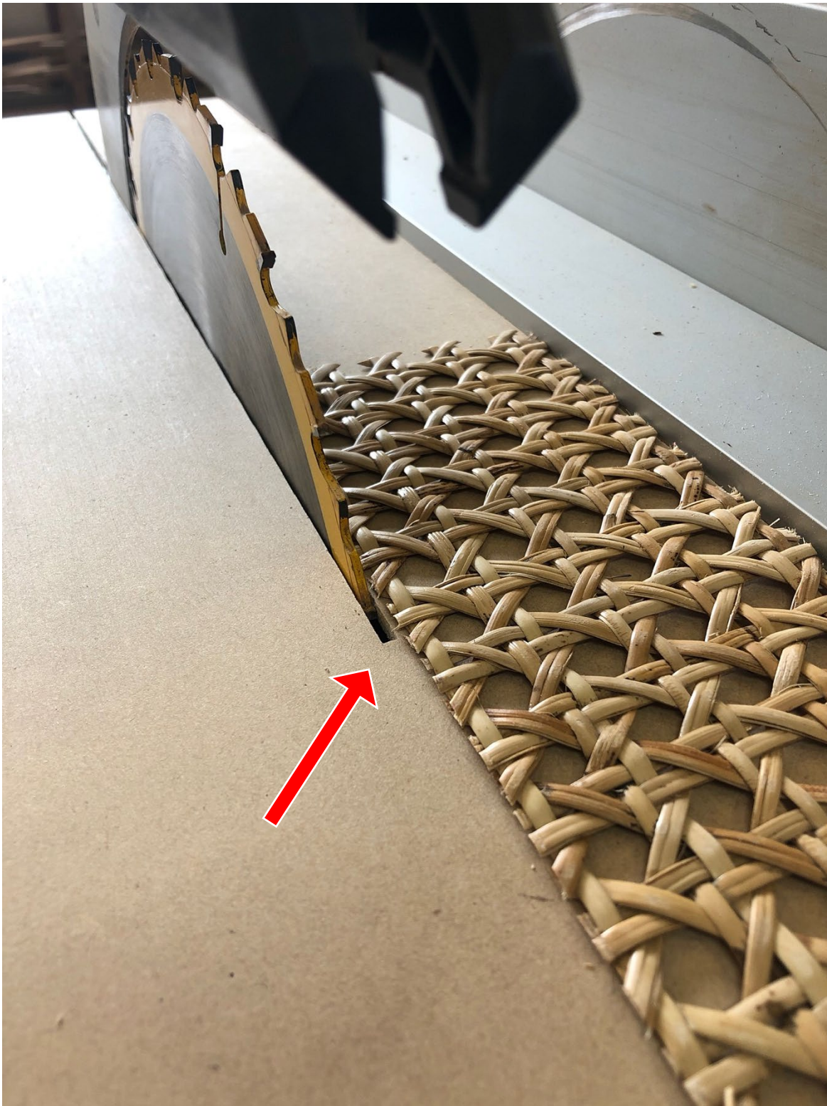
Figure 41. A sacrificial cover sheet (width of the saw blade) on top of the infeed table reduces the gap in the table. This guarantees a safer work process and higher quality of sample edges
