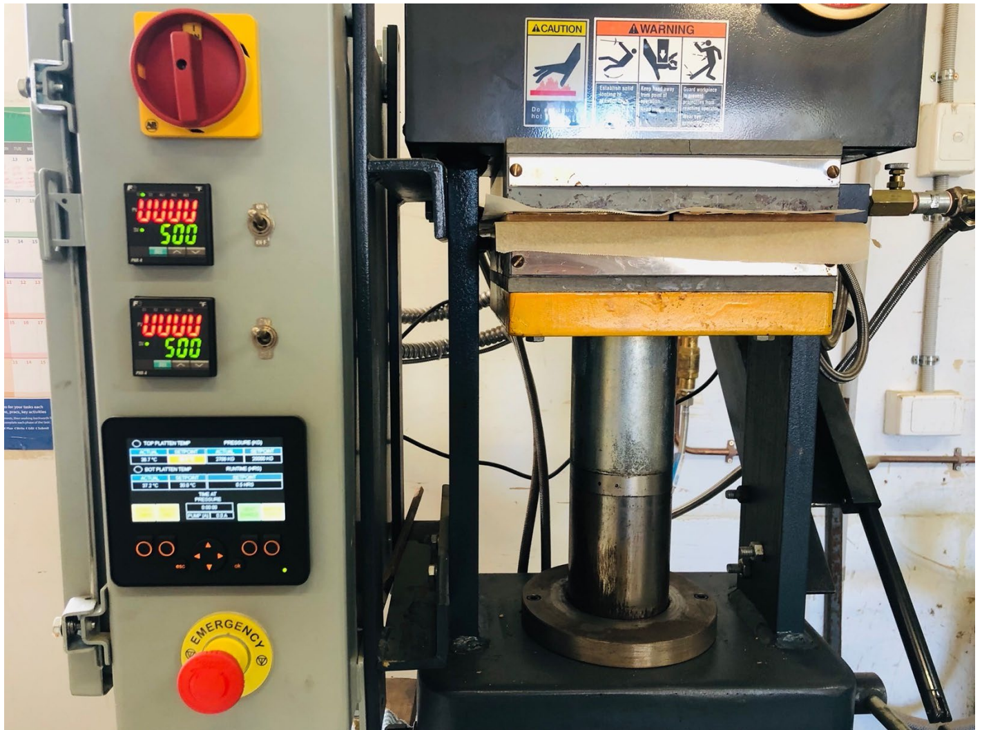
Figure 50. Sample assembly in the laboratory press (Dake model 944226, USA).
