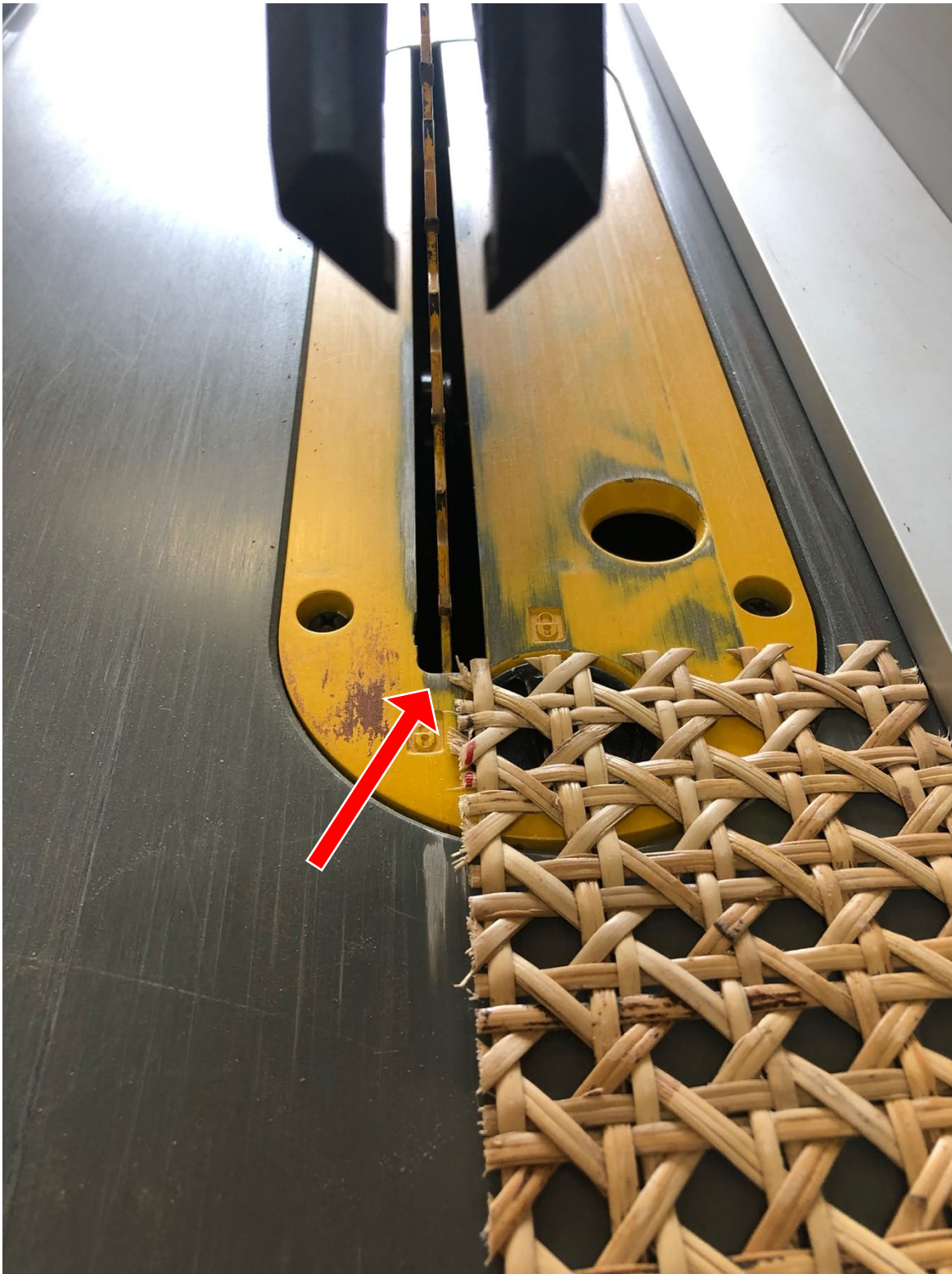
Figure 40. A large gap in the infeed table of the table saw can cause rough edges and disintegration of mats especially with loose weaving.
