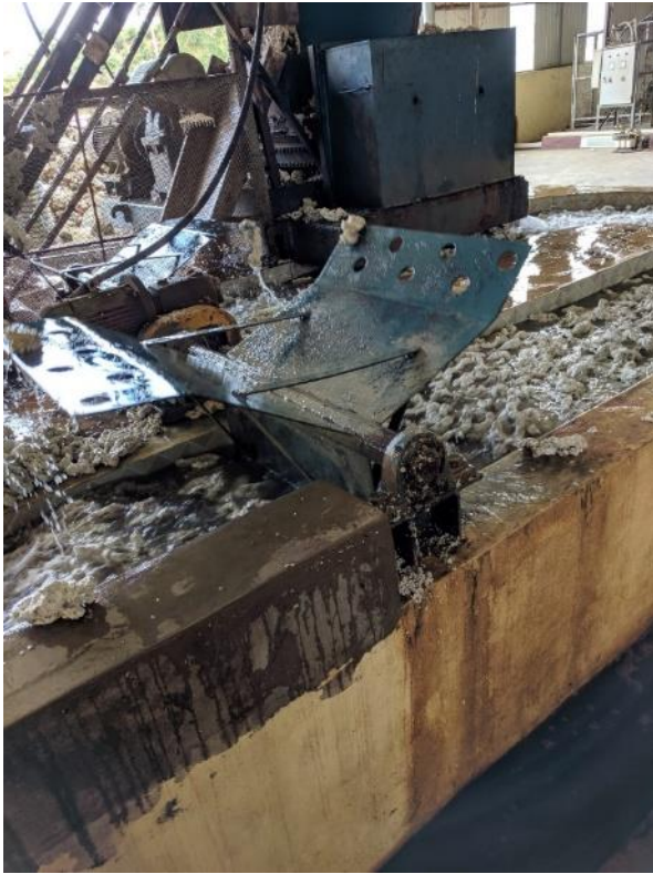
Figure 17: Cup lump washing and shredding
