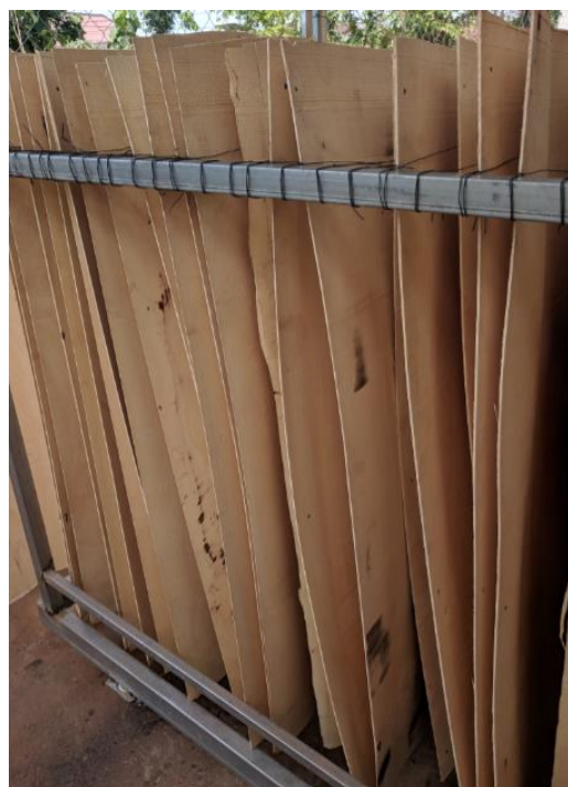
Figure 25: Rubberwood Veneer peeled at NUoL
