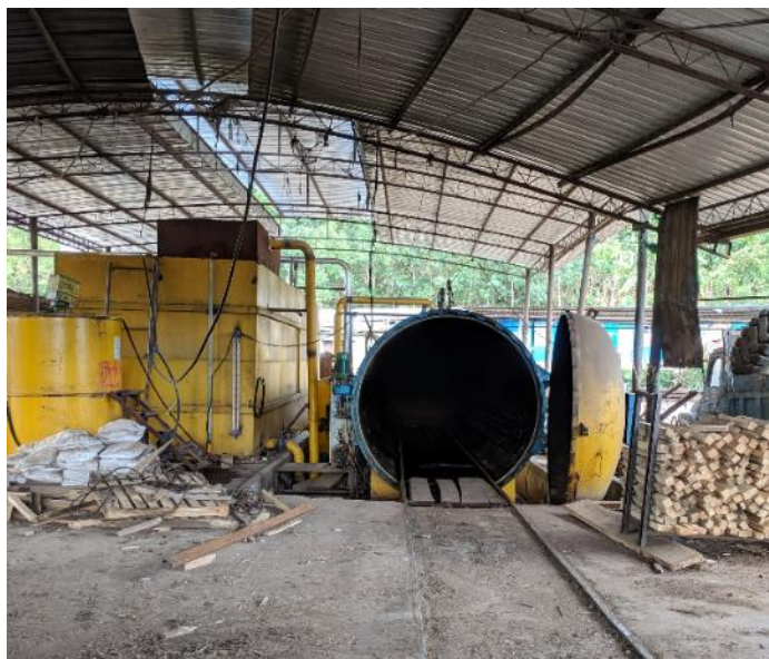
Figure 26: Pressure treating rubberwood for fungal decay
