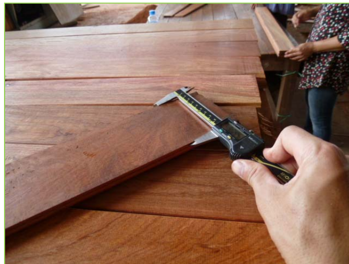
Figure 10 Measuring the pieces after a processing step to assess variation and make sure that the machine is calibrated will increase productivity and reduce wood waste.
