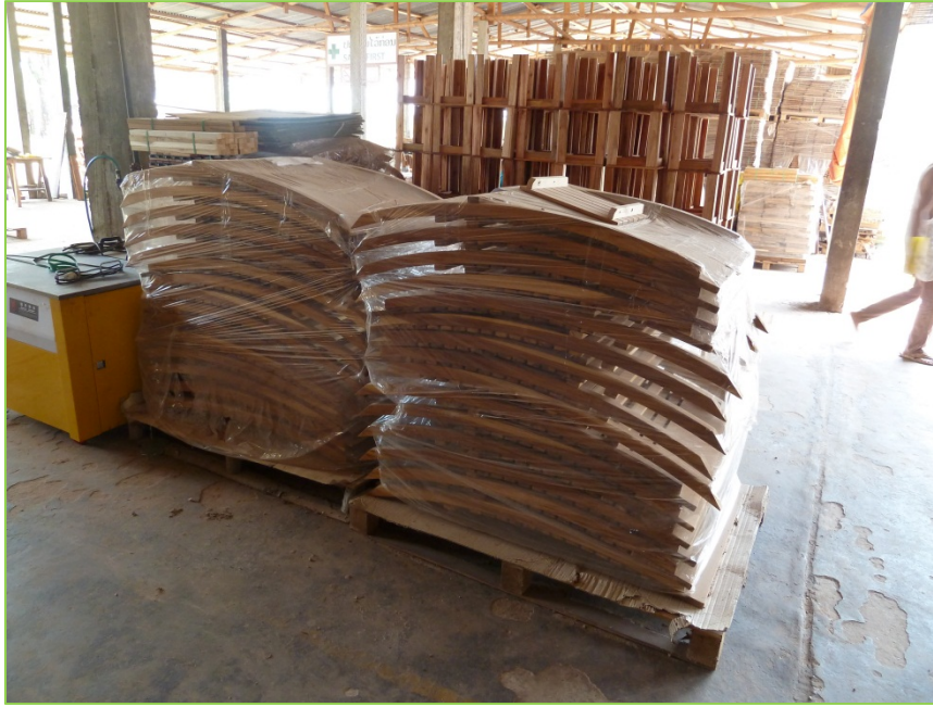
Figure 14 Wrapping finished products will reduce the risks of degrading them prior shipping.
