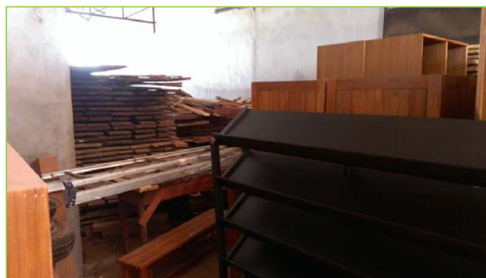
Figure 4 Inappropriate storage can damage lumber and cause production delay while reducing storage space.
