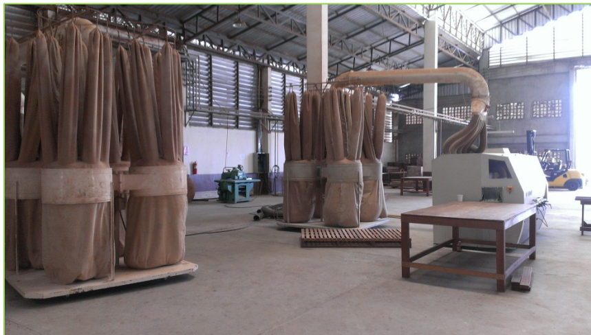
Figure 20 Having an exhaust system will not only provide a safe and healthy working environment but also simplify maintenance and increase productivity and product quality.
