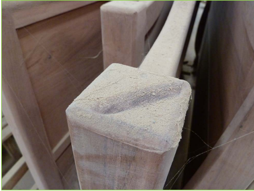
Figure 18 Wood dust adds an extra step in the process because components need to be cleaned before finishing otherwise this will affect the quality of the finish and subsequently of the wood product.
