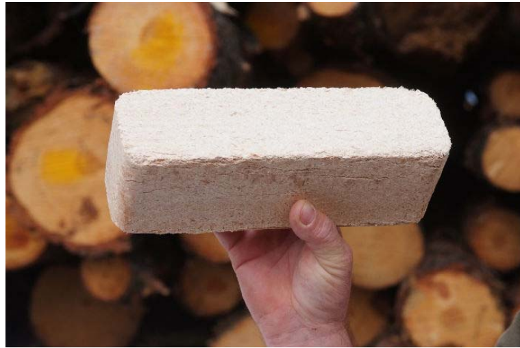
Figure 24 Brick made from sawdust ( www.sourceable.net ).
