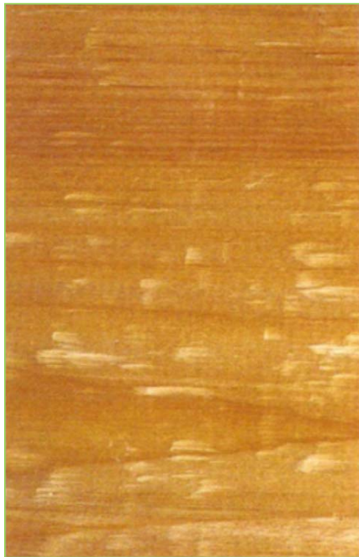
Figure 19 Chip marks are the result when a machine's exhaust system isn't capable of clearing debris from the cutterhead. This will require additional sanding and increase your processing costs.
