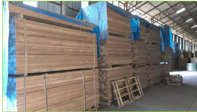
Figure 3 Kiln dried lumbers stored in an enclosed dry shed and covered with a waterproof tarpaulin will prevent deterioration.
