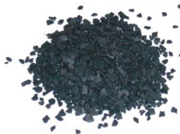
Figure 25 Activated carbon is an adsorbent for gaseous contaminants in many industrial applications.
