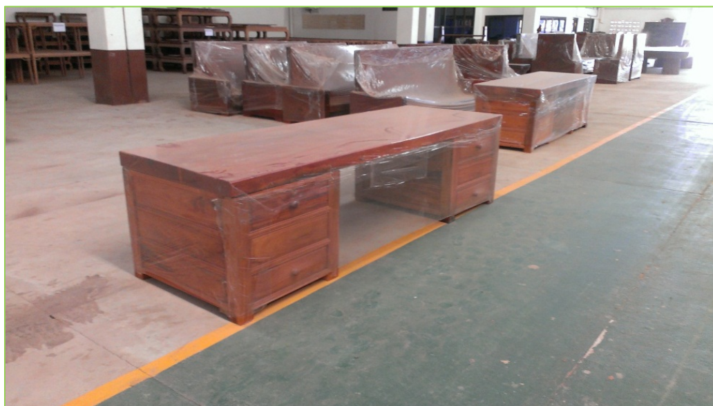
Figure 13 Wrapping finished products will reduce the risks of degrading them prior shipping.
