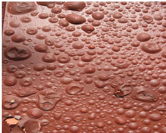
Figure 23: Cissing problem (reproduced from http://voices.yahoo.com/how-fix-common-paint-faults-11860425.html?cat=30 )
