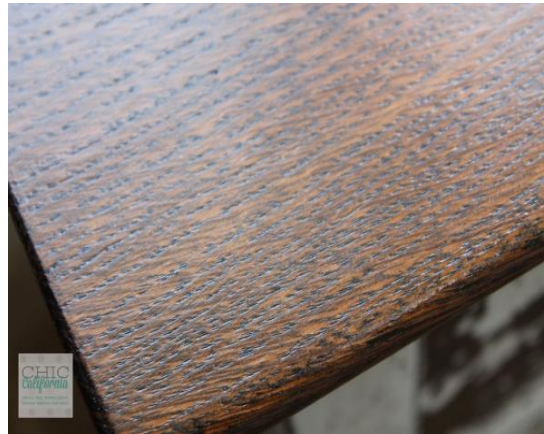
Figure 22: White-in-the-grain finish problem (reproduced from http://chiccalifornia.com )
