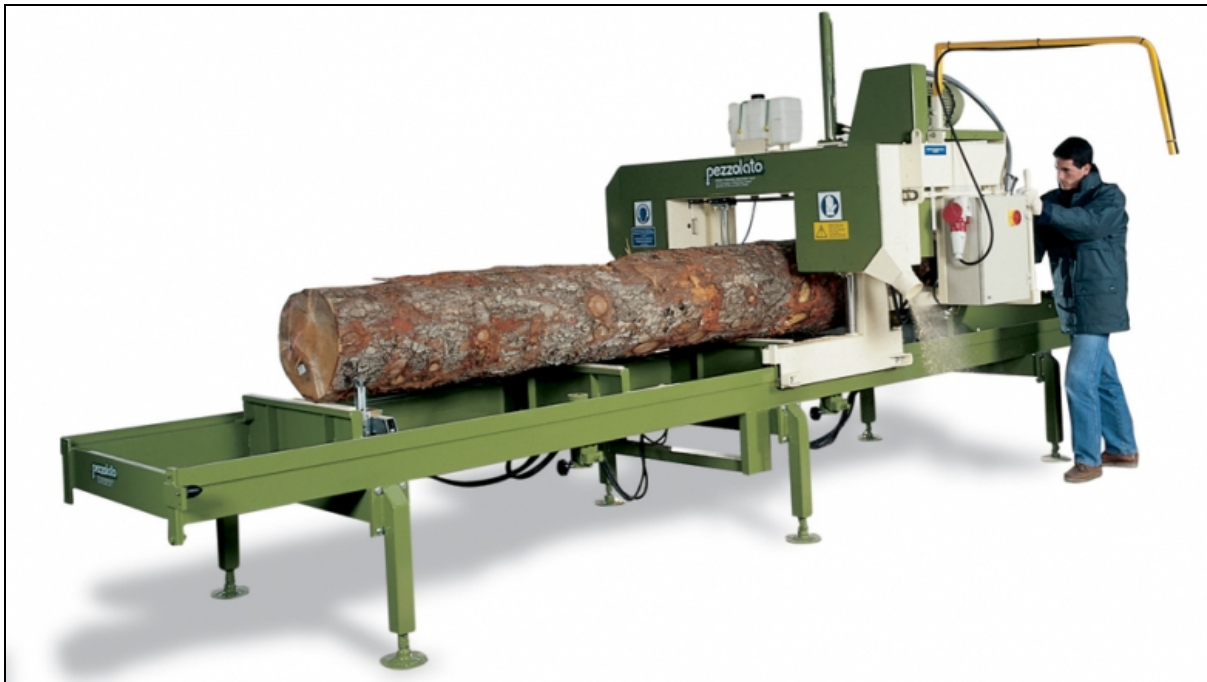
Figure 10: Pezzolato Timber Queen HD 7 portable band sawmill ( www.pezzolato.it )
