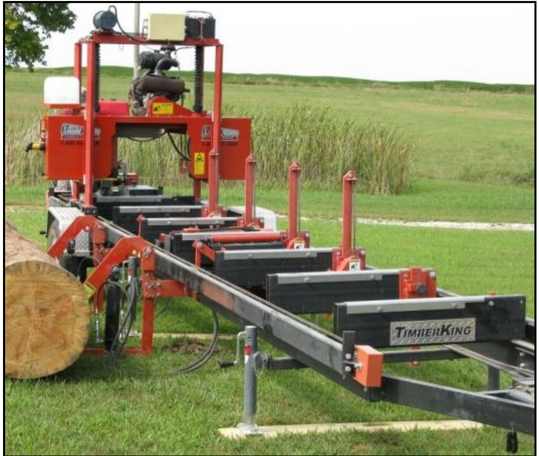
Figure 12: TimberKing 2000 portable band sawmill ( www.timberking.com )
