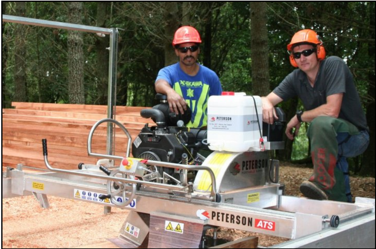
Figure 14: Peterson ATS portable circular saw – swingblade sawmill ( www.petersonsawmills.com )
