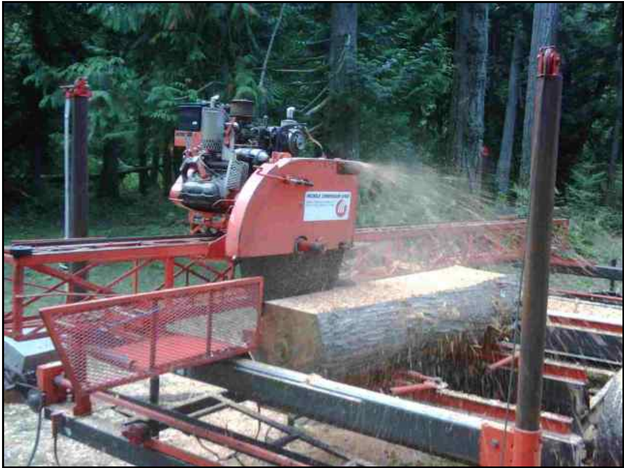
Figure 4: Mobile Mfg. portable mobile dimension sawmill ( www.mobilemfg.com )
