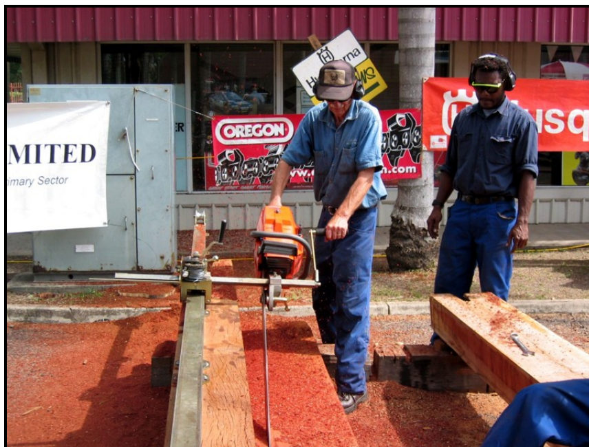
Figure 1: A Westford chainsaw mill ( www.westformills.com.au )
