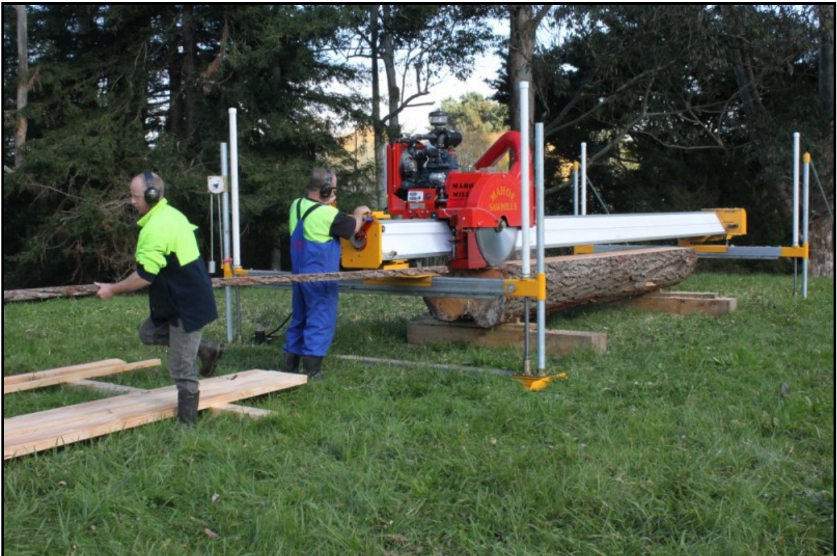
Figure 14: Mahoe Supermill portable circular blade sawmill ( www.sawmills.co.nz )
