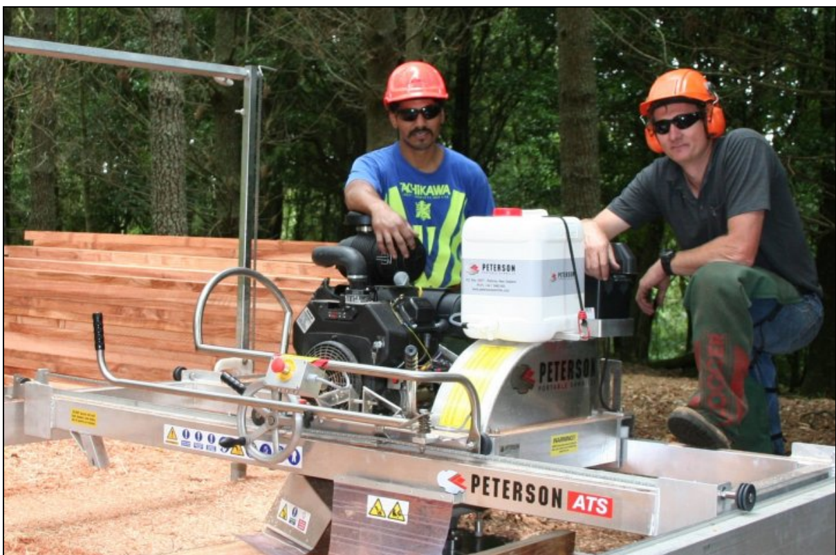
Figure 3: Peterson Sawmills ATS portable circular swing blade sawmill ( www.petersonsawmills.com )
