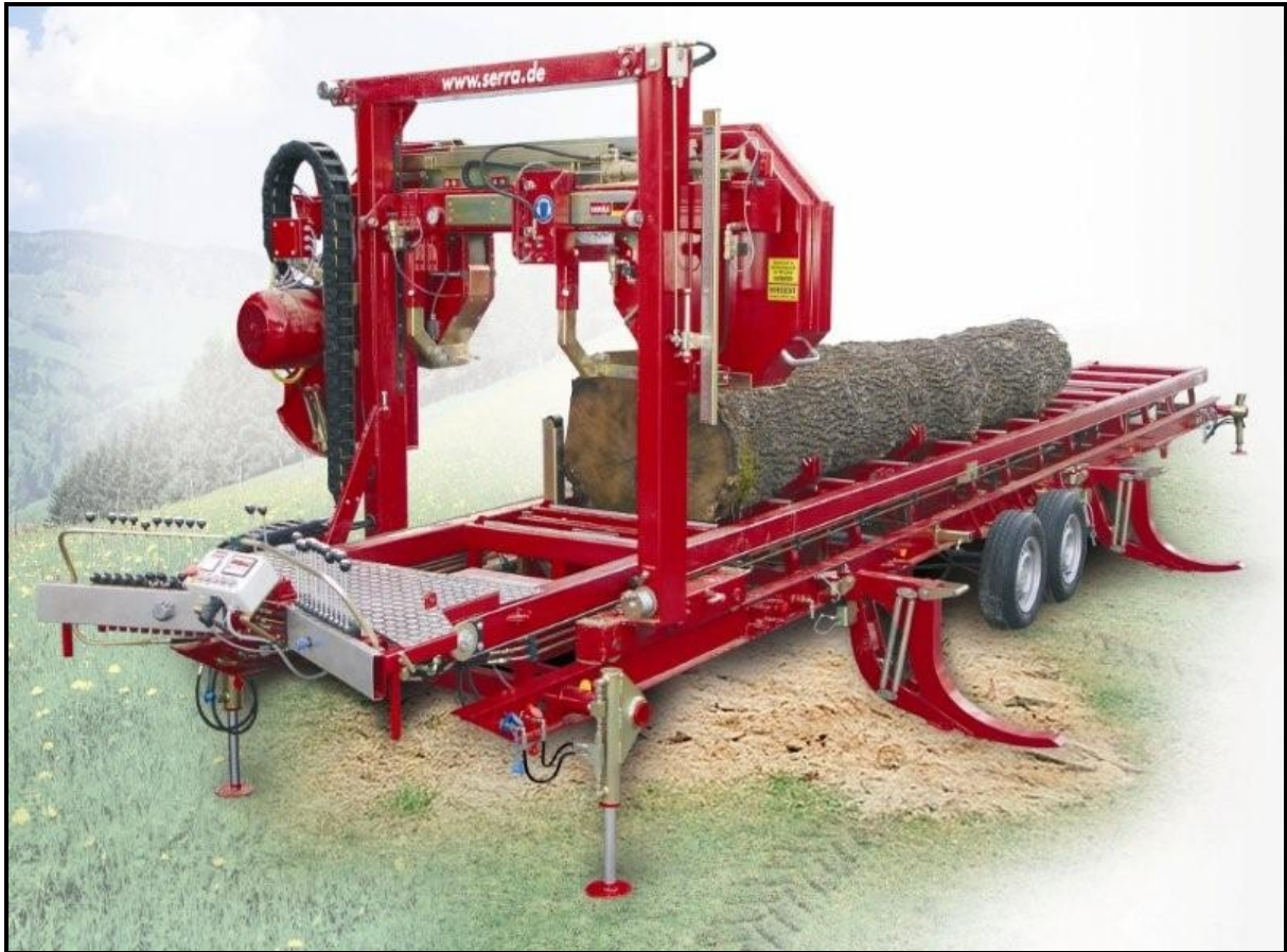
Figure 7: Serra Alpina KE90 portable band sawmill ( www.serra.de )
