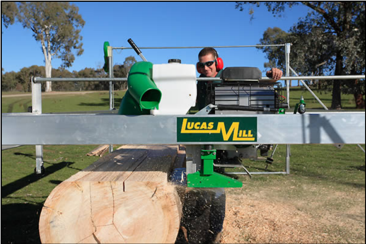
Figure 13: Lucas Mill portable circular saw - swingblade sawmill ( www.lucasmill.com )
