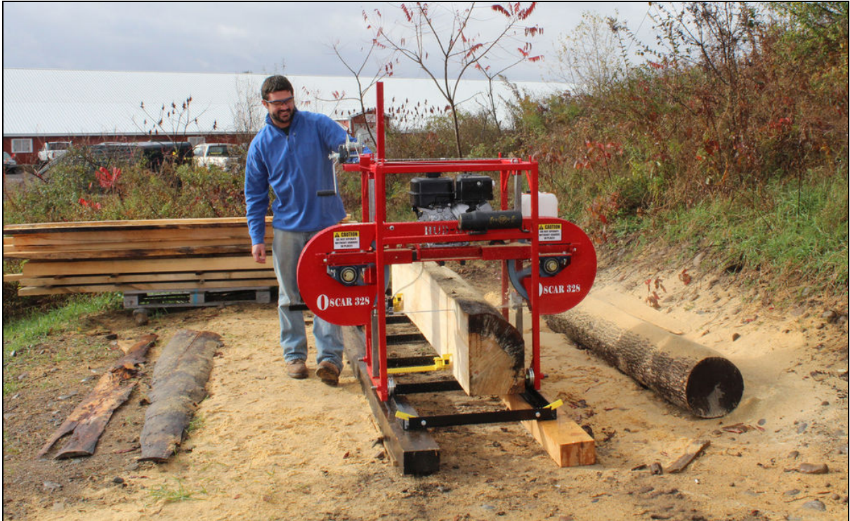
Figure 11: Hud-Son Oscar 121 portable band sawmill ( www.hud-son.com )
