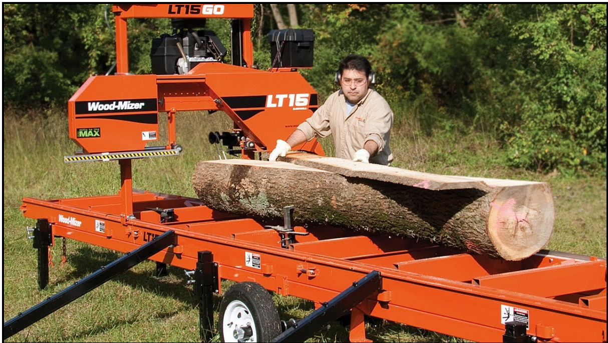
Figure 6: Wood-Mizer LT 15 portable band sawmill ( www.woodmizer.de )
