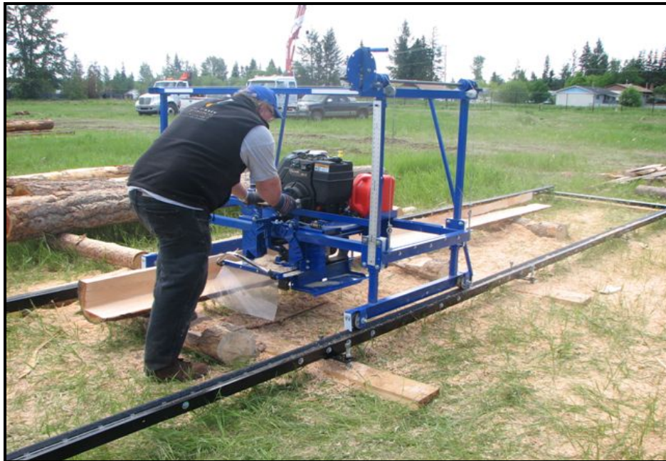
Figure 15: D & L Timber Technologies portable circular swingblade sawmill ( www.dltimbertech.com )
