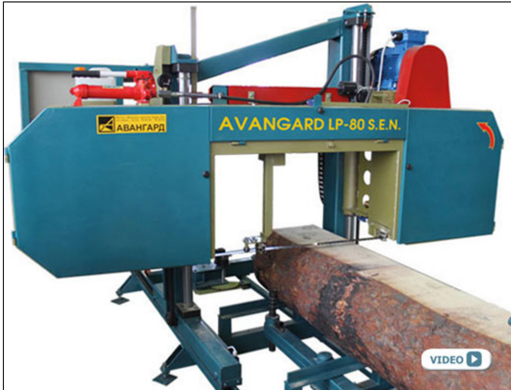
Figure 9: Avangard LP-80 S.E.N. portable band sawmill ( www.pilorama.ru )
