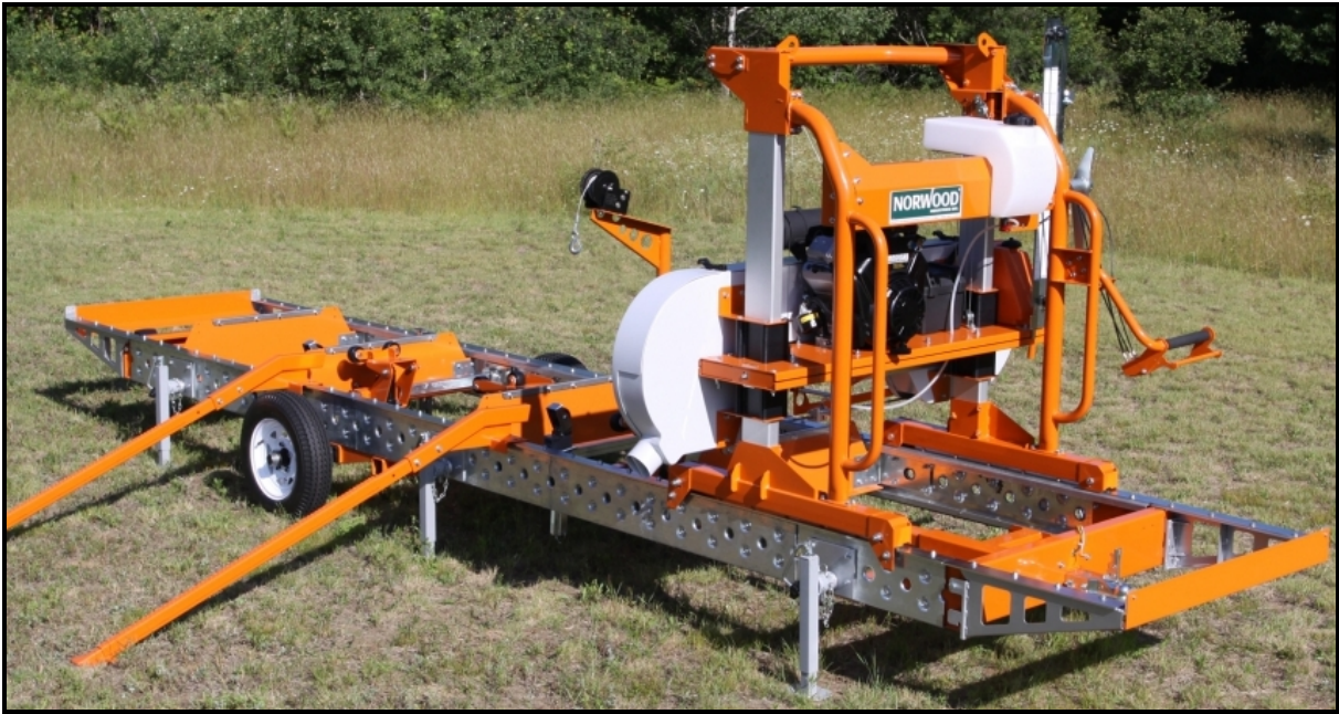
Figure 8: Norwood LumberMate Pro portable band sawmill ( www.logosol.de )
