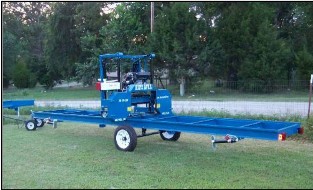
Figure 5. Enercraft-Baker 18M portable band sawmill ( www.baker-online.com )
